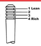
1 = Without Rotax® intake silencer kit, with K&N RC1200 air filter, with or without Rotax® after muffler kit.
