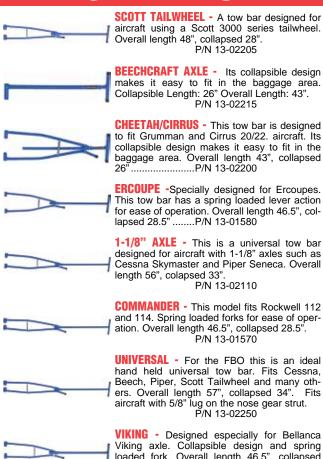
VIKING - Designed especially for Bellanca Viking axle. Collapsible design and spring loaded fork. Overall length 46.5", collapsed 28.5" ......P/N 13-02220
