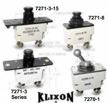
The Klixon 7270/7271 series circuit breakers were designed to utilize less behind panel space while protecting wire and cable in aircraft and ground support equipment on either 120 VAC, 400 Hz or 30 VDC systems. The units are available with neck mounting (7270-1 and 7271-8) or standard cover plate (7270-7 and 7271-3). In each of these Klixon circuit breakers, the bi-metallic element assures uniform current distribution
