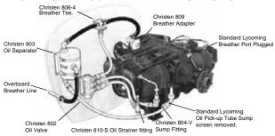
This accessory kit for Lycoming engines provides normal engine lubrication with minimal oil loss during aerobatic flight. It functions as a selfcontained extension of the normal engine oil and breather systems. Can be installed in a few hours without engine disassembly.
