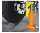
The pad is available without the remote bottle jack. The 30M-B90 Jack Pad is bottle jack. The 30M-B90 Jack Pau is great for raising one wheel for a tire change, repacking wheel bearings or servicing the brakes. When used with a long stroke jack, the jack pad may be used to change a flat tire. Small and light enough to carry on board, the jack pad adds mission capability when operating from airports that do not have full service or wing jacks large enough to lift these aircraft
