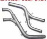
Replacement mufflers & exhaust components for Luscombe/Ercoupe Aircraft, all are FAA/PMA approved equivalents.
