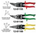
Famous for cutting ease, keeping their edge and making clean, sharp cuts. Hardened molybdenum steel blades, serrated jaws and vinyl comfort grips. Capacity 18 gauge (.049") steel. Length 9-3/4". Wt. 14 oz.
