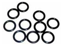
Fluorocarbon rubber o-rings. Fluorocarbon rubber is commonly known as Viton. It is an advanced rubber that has extremely good fuel and heat resistance and is ideally suited for aircraft fuel system applications.
