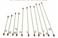
APS® offers stainless steel fuel injection lines for use with many of the popular Lycoming RSA style fuel injection assemblies. APS® stainless steel fuel injection line assemblies are manufactured to extreme standards and are 100% pressure tested at 80 psi for leaks.
