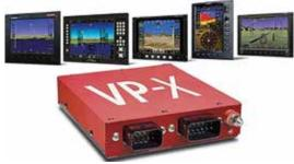
The VP-X integrates with many popular EFIS products enabling you to monitor and control your entire electrical system on the EFIS display. In addition using the EFIS for attitude, navigation, and engine information, you now can use the EFIS display to monitor the health of your electrical system, view and control the status of individual circuits, and respond to circuit faults.
