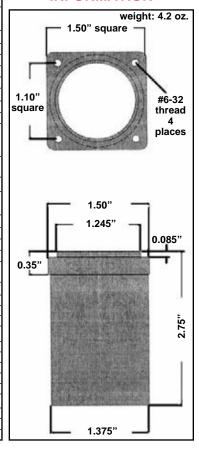
These 1 1/4" instruments are identical to the 1 1/4" UMA Gauges on previous page, except these are TSO'd for certified aircraft. (Except Ammeters)
