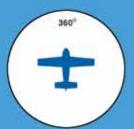
strobe light system must project light 360° around the aircraft's vertical axis. One or more strobe lights can be used.
