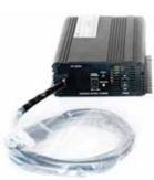
MODEL JAC2024H - Intelligent chargers follow battery impedance to end of charge cycle for all battery types. Fully automatic. Green LED indicates AC power on, yellow LED indicates battery is charging, yellow LED off indicates float mode. Charge control: constant current charge to a constant voltage, then to a float standby. Current limiting. Fully automatic 3 stage charger can be left on the battery in maintaining/float mode. Can be set for any type lead acid battery,
