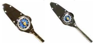
Dial Type Wrenches provide unmatched reliability, accuracy and durability for applications where torque measurement is extrememly critical. Models feature a memory pointer that indicates the highest torque achieved during application of torque. 2% accuracy clockwise and counterclockwise. All wrenches are made in the USA of all steel construction for the highest quality. Both models come with a plastic storage box and a calibration compliance certificate.
