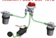
These systems have a PX375-TC Fuel Boost Pump either for 3/8" or 1/2" fuel lines and GAS375 Gascolator, Some kits may have two Gascolators: one with the standard flow direction (Right to Left) and one with the reverse flow (Left to Right), mounted in the wing roots.
