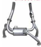
P/N 08-02100-Fits Lycoming O-320 (Vertical Induction Intake) (Must use "short" miniature light weight Sky Tec starter for clearance) (Optional studding to increase cabin heat available)
