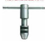
General's Reversible Tap Wrenches feature a fine-tooth ratcheting mechanism which adjusts on the fly for right - and left-hand use. In addition, the ratchet can be locked to transform the tool into a standard tap wrench. The self-centering, hardened-steel jaws assure the formation of straight threads in your work piece. Although designed mainly for holding taps, the Reversible Tap Wrench also works great with reamers, drill bits, screw extractors and other hand-turned tools.
